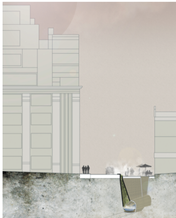
Ray Street: the Fleet sewer jumps down 1 m due to its location on the Thames River terrace.
