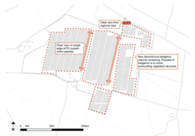
The use of a discontinuous hedgerow at Solarfeld Gansdorf aims to reduce the visibility of the solar field and at the same time mimic the appearance of the surrounding landscape structure.
