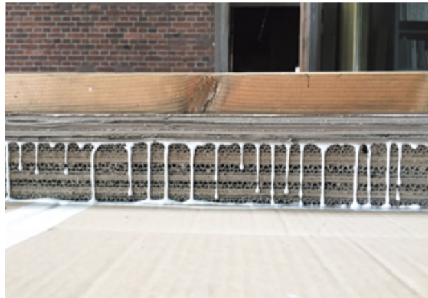
Cardboard processing. Gluing and pressing leftover cardboard creates a strong building material.
