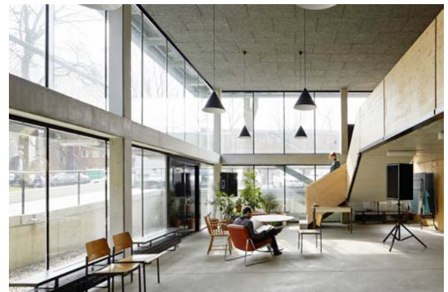
Double-height shared space, legally considered a winter garden (thereby allowing the double-height glazing) in R50 Baugruppen project in Berlin (image via Metropolis.) This shared space features a gallery-level guest room, whilst also affording potential adaptation into two levels, as required. Baugruppen often seems to exemplify adaptive design.
